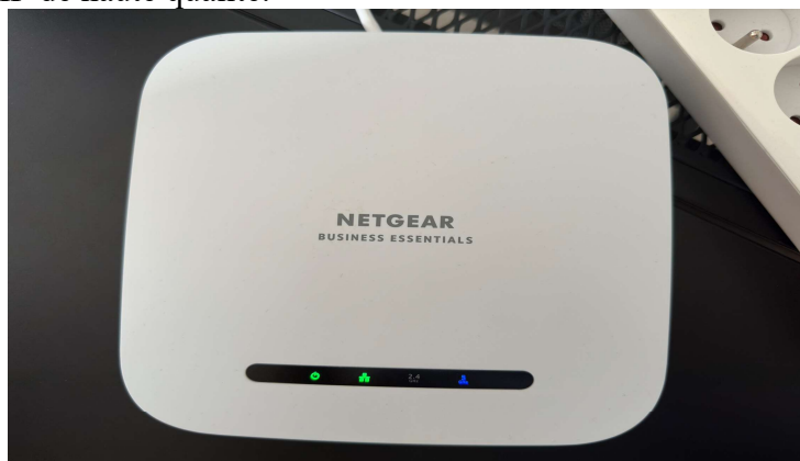
Figure 5 : Borne wifi NETGEAR ( WIFI 6 AX1800 Dual-band Access Point with PoE WAX214V2)
